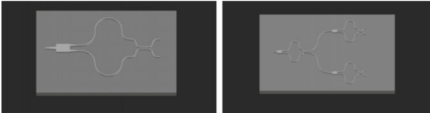
Fig. 1 The schematic layout of the proposed CWDM (de)multiplexer
