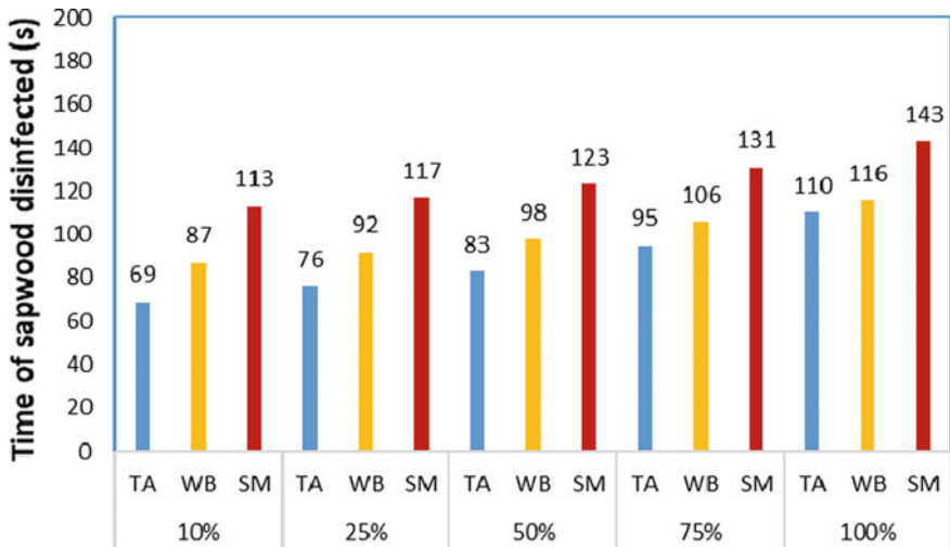
Fig. 13 Heat treatment by microwave energy ( I_0 = 1 \text{ W/cm}^2 , f = 2466 \text{ MHz} ): Evolution of percentage sapwood disinfected (initial temperature is 0 \text{ }^\circ\text{C} )
