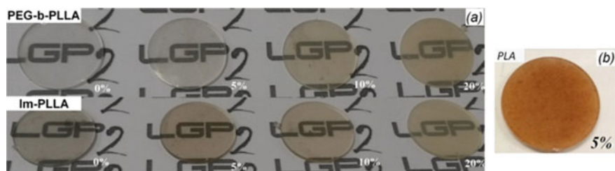
Fig. 7 Effect of adding various levels of modified surfactants onto PLA and injection molded into discs a and image of unmodified PLA composites (Mariano et al. 2017). Reproduced with permission from American Chemical Society through open access publishing
