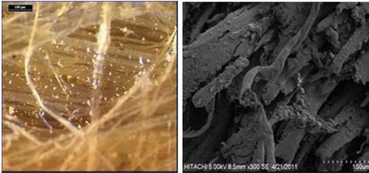
Fig. 4 Misaligned of fibres (Suriani et al. 2012)
