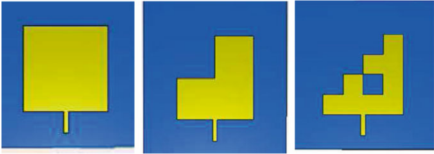
Fig. 1 The geometry of simulated Sierpinski step-shaped fractal reference square patch for two iterations
