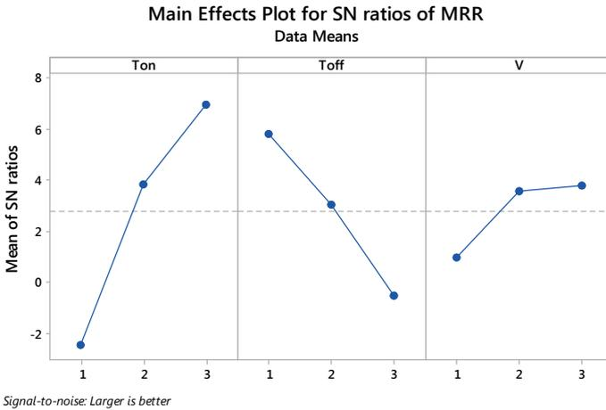
Fig. 2 Effect of parameters on MRR
