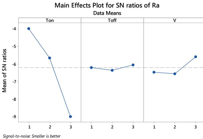
**Fig. 3** Variation of S/N ratio with selected parameters for Ra
