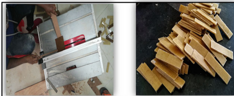
Fig. 4 Specimens cutting preparation by power circular saw machine
