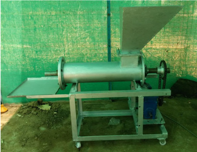
Fig. 3 Front view of fabricated pellet machine
