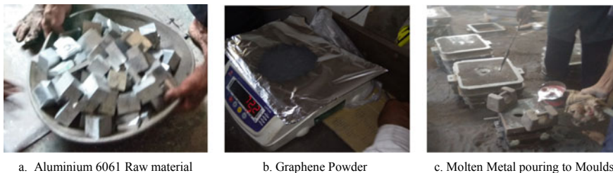
Fig. 1 Material casting process
