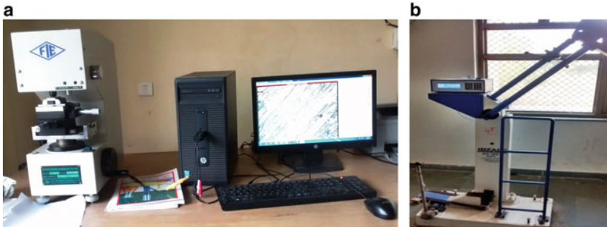
Fig. 4 a Micro Vickers hardness test, b Impact testing machine
