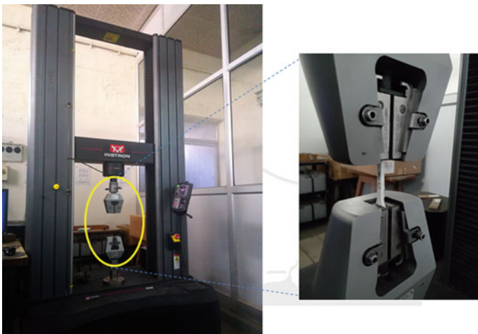
Fig. 3 Tensile testing of 3D-printed samples
