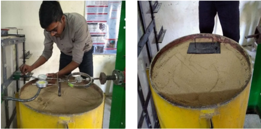
Fig. 3 Laboratory Test setup for lateral load
