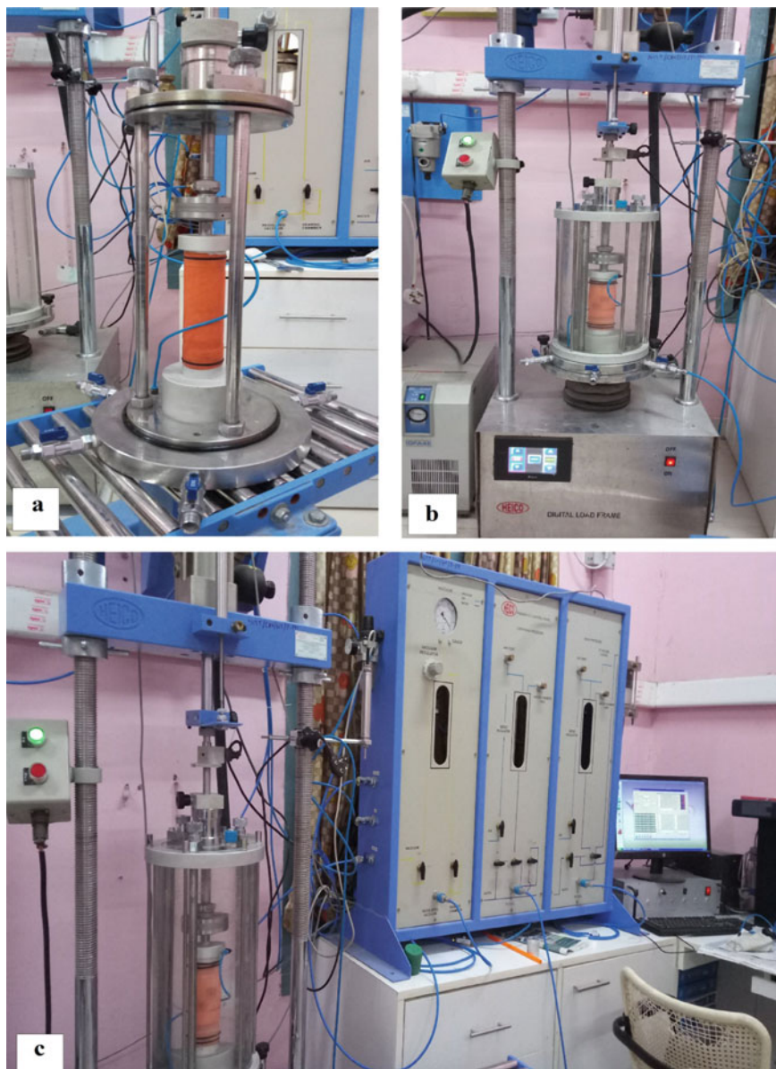
Fig. 2 Triaxial test of LSS-ISAC-1. a Sample preparation, b confining chamber with sample, c loading assembly of triaxial test
