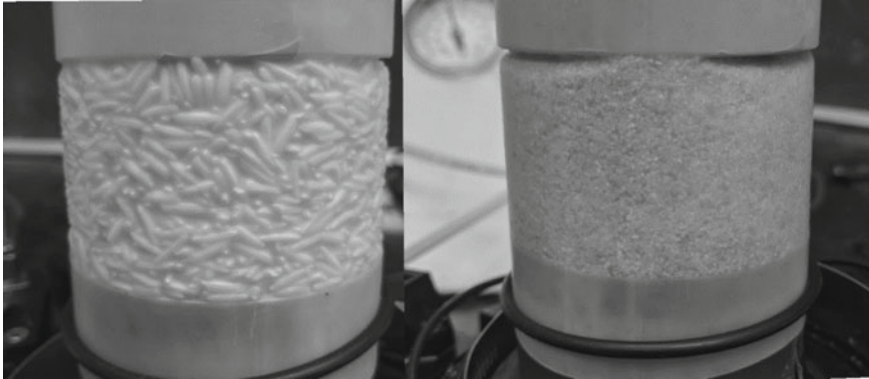
Fig. 3 Prepared sample at 60 kPa for rice (Left) and monterey sand (Right)
