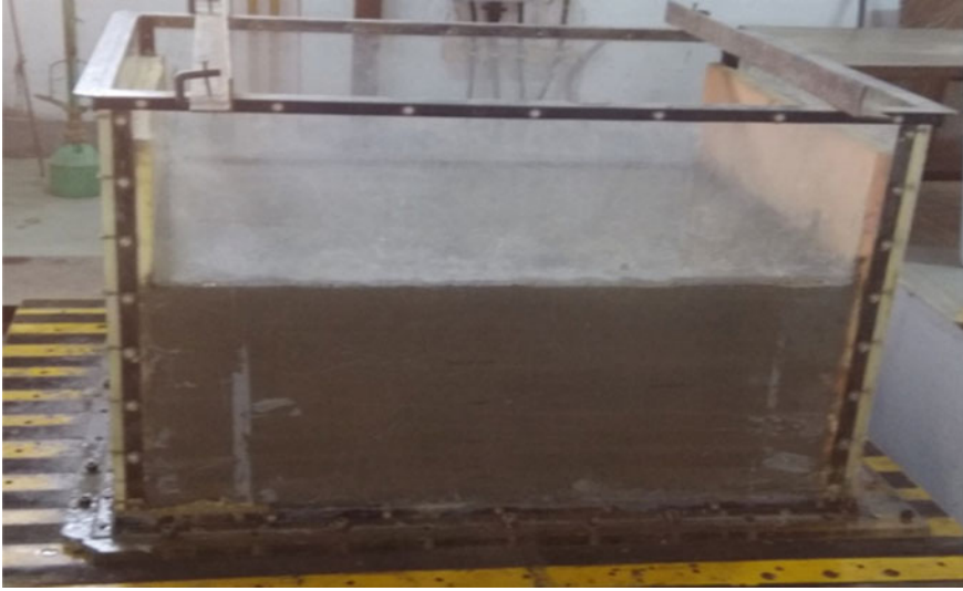
Fig. 1 Prepared sand bed for the desired relative density
