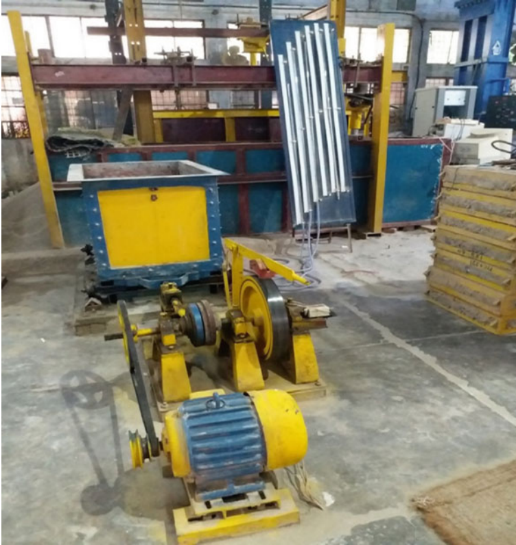
Fig. 1 Shake table test set up used in the study
