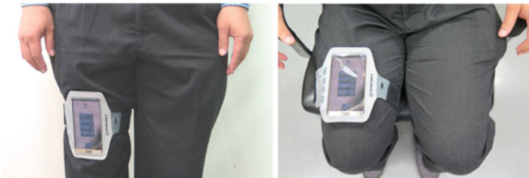
Fig. 2 Position of the smartphone on the thigh
