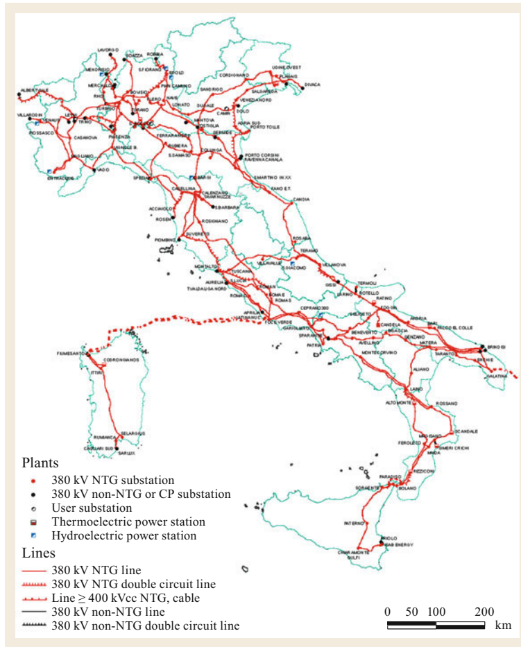
Fig. 5.13 Italian 380 kV network on 31.12.2018 ( https://www.terna.it )
