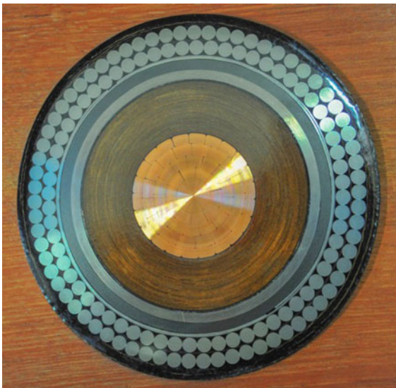
Fig. 10.53 Cross-section of a mass-impregnated cable (adapted from [10.6])
