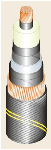
Fig. 10.76 Example of a single-core cable design (adapted from [10.39])
