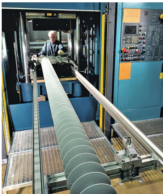
Fig. 9.96 Injection molding of a 420-kV SR composite insulator using the stepping technology (source Pfisterer Sefag)
