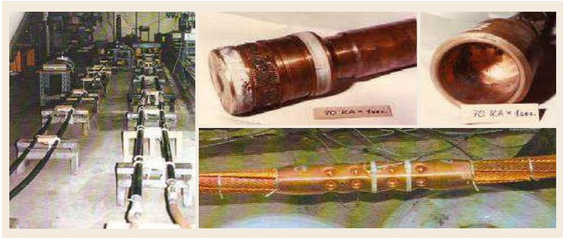
Fig. 10.111 Tests of connectors (adapted from [10.49])
