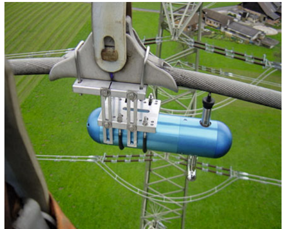
Fig. 9.59 Modern vibration recorder in the field (photo: Pfisterer Sefag)
