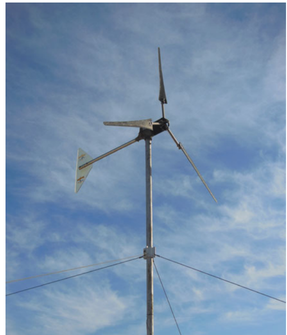
Fig. 15.12 A small horizontal-axis wind turbine installed at the Electric Energy Systems Laboratory of the National Technical University of Athens (Courtesy Authors)
