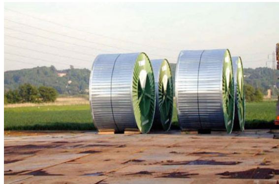
Fig. 10.5 Typical cable drums for 400 kV cables (adapted from [10.8])
