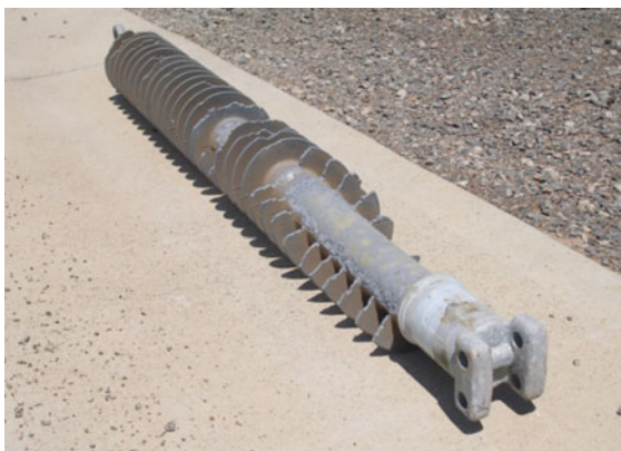
Fig. 11.34 Bird damage on a composite insulator (Courtesy TransGrid, Australia)
