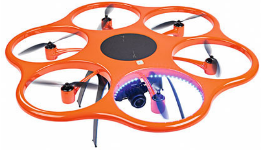
Fig. 9.173 UAV with propeller side protection and camera for visual inspections (adapted from [9.277])
