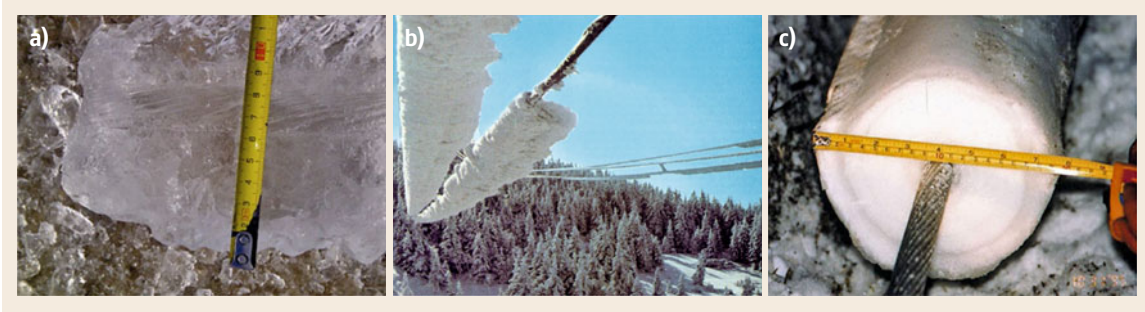
Fig. 9.14a–c Different types of ice on conductors. (a) Glaze ice (photo: F. Jackl), (b) soft rime, (c) wet snow (photo: Landsnet, Iceland)
