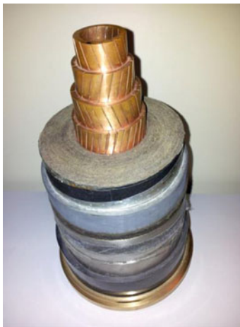
Fig. 10.56 500 kV SCFF cable with a 1600 mm 2 copper keystone conductor and a lead sheath (adapted from [10.42])
