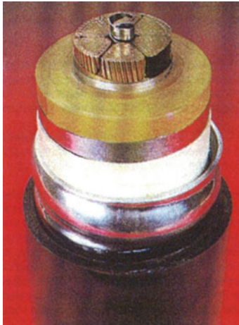
Fig. 10.55 400 kV SCFF cable with a Milliken copper conductor and a corrugated aluminum sheath (note the helical duct support) (adapted from [10.42])
