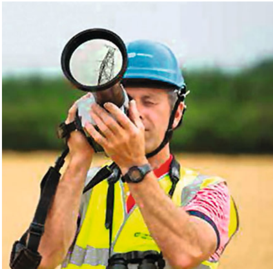
Fig. 9.171 Thermographic joint inspection performed from the ground (adapted from [9.271])
