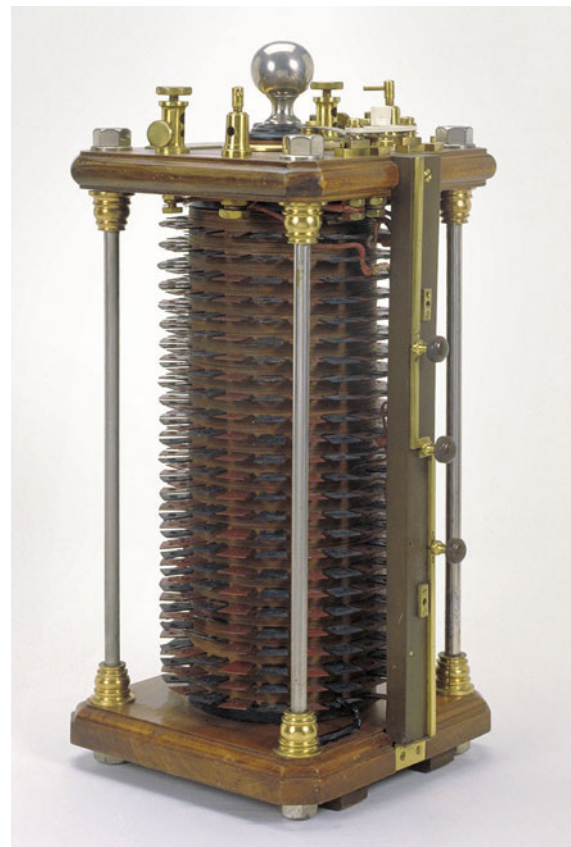
Fig. 7.2 Model in the Museo Galileo (Florence, Italy) of the transformer constructed by Gaulard and Gibbs [7.4]
