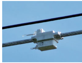
Fig. 9.47 Monitoring through vibration analysis (adapted from [9.96])
