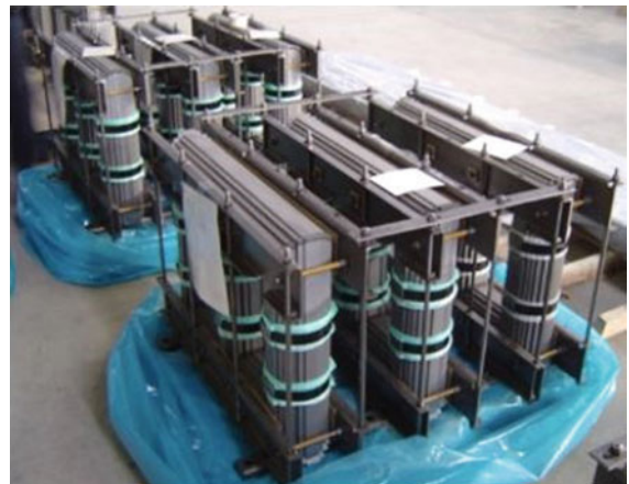
Fig. 7.41 Transformer cores with step-lap and outer tie rods [7.24]
