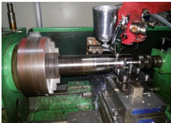
Fig. 2 Minimal quantity lubrication setup and spray gun
