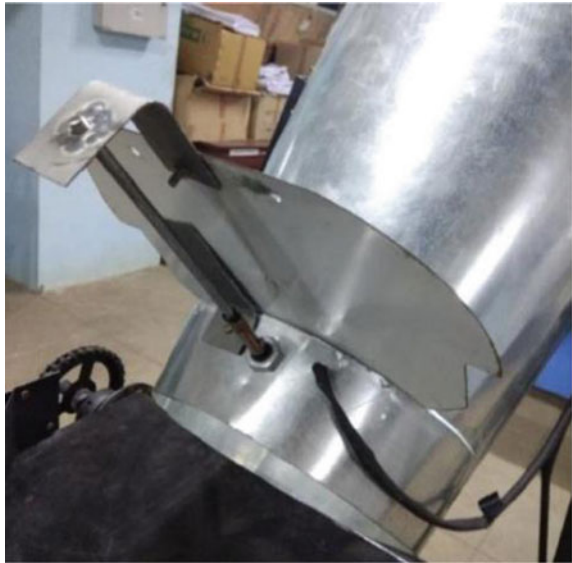
Fig. 3 Waste flow control mechanism
