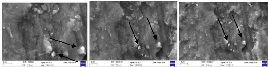
Fig. 3 Micrograph of Al6061 + 3% of TiB 2 with 15KX, 10KX, and 7.5KX
