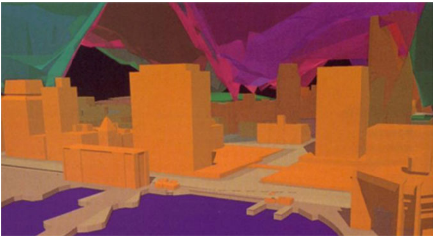
Fig. 16.4 Sunlight control modeling for Auckland city (1988), with the operative envelopes visualized as “stained glass” windows (Cadabra)
