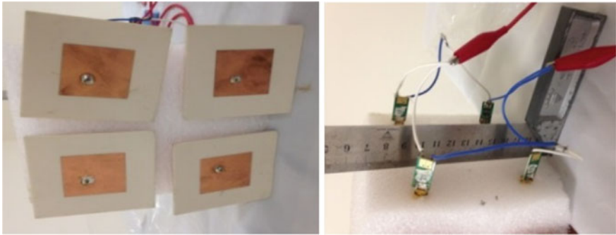
Fig. 2 Receiving antenna array and attached rectifier circuit configuration
