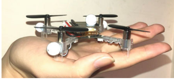
Fig. 1 The palm-sized nanoquadcopter, Crazyflie 2.0, attached with reflective markers
