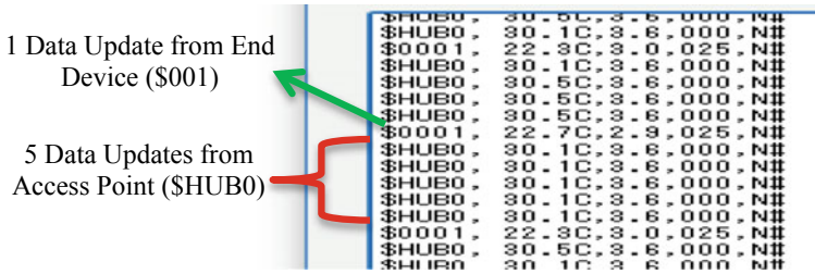
Fig. 4 Configured sensor tag readings on sensor monitor application console
