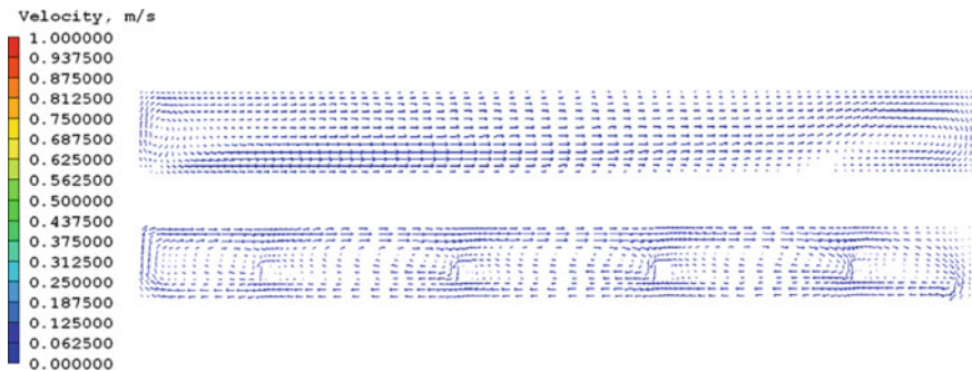
Fig. 9.8 Velocity vectors at the middle cross-section beneath photovoltaic module for natural convection (top) and heat recovery (bottom)
