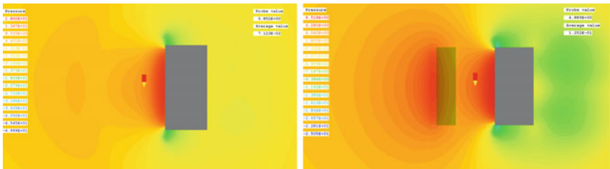
Fig. 1.12 Predicted pressure contours at the middle plane (XY) of the building ( Z = 4 m) without trees (left) and with trees at D = 8 m from the building (right)
