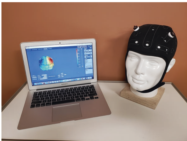
Fig. 18.2 Transcranial Direct Current Stimulation (tDCS) device Starstim 8 5G, from Neuroelectronics. Picture taken at the Laboratory for Neuropsychiatry & Neuromodulation, Division of Neuropsychiatry, Department of Psychiatry, Massachusetts General Hospital. Courtesy of Dr. Patricia Cirillo and Prof. Joan Camprodon
