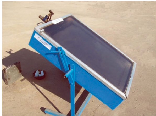
Fig. 11.8 Solar wax melting device (Source: Chaurasia, 1991)
