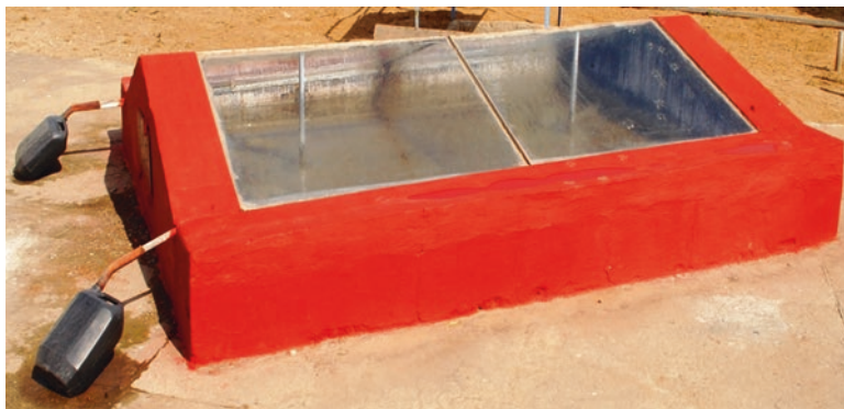
Fig. 11.9 Solar desalination devices made of vermiculite-cement material. (Source: CAZRI Annual Report 2013–14, pp. 87)
