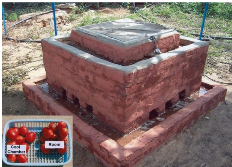
Fig. 11.10 Improved zero energy passive cool chamber for preservation of vegetables. (Source: Chaurasia et al. 2005)
