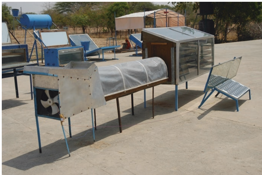
Fig. 11.5 PV winnower-cum-solar dryer. (Source: Pande 2006)
