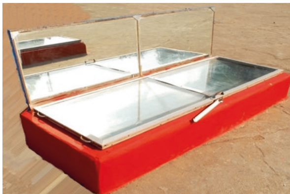
Fig. 11.7 Solar cooker for animal feed with reflector. (Source: Nahar 1994)
