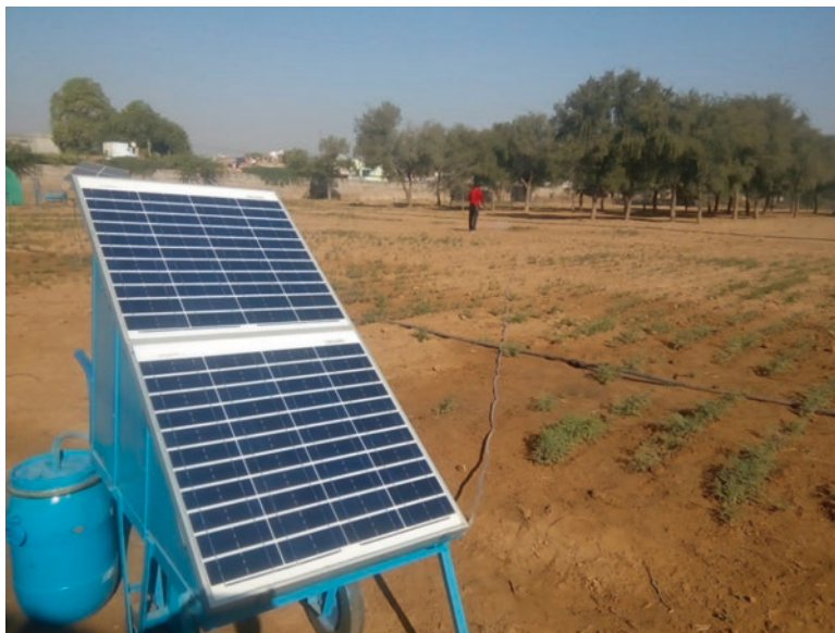
Fig. 11.2 Solar PV sprayer. (Source: CAZRI Annual Report 2016–17, pp. 98–100)
