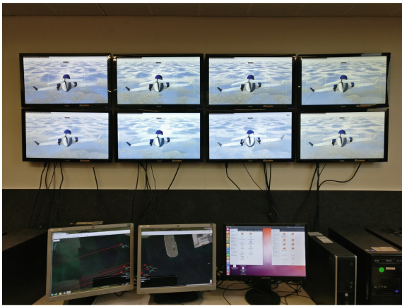
Fig. 1. The flight gear cluster simulator simulating a search and rescue operation with eight UAVs
