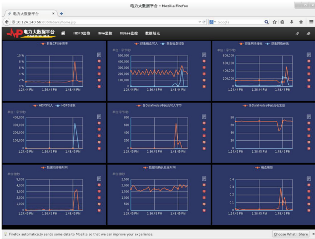
Fig. 2. User interface of operational and maintenance system for power grid Big Data platform
