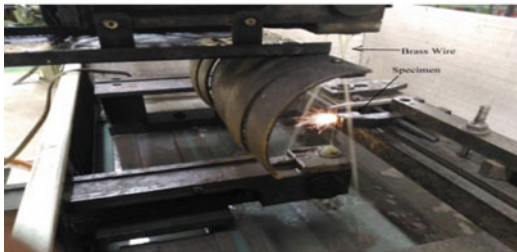
Fig. 60.3 a. WEDM setup with CMC b. WEDM cut (9 cuts) on specimen
