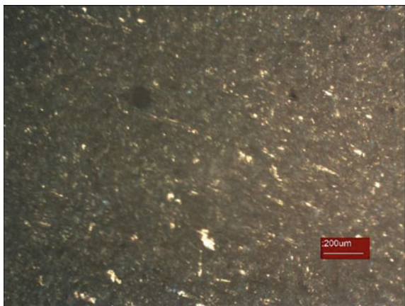
Fig. 11.8 Optical microscopic images at WP = 320 MPa, AFR = 0.64 kg/min, and SOD = 1 mm
