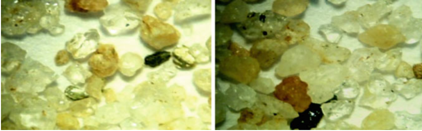
Fig. 14.17 Silica sand of 425 \mu\text{m} before and after machining respectively
