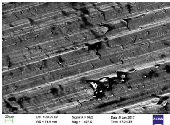
Fig. 9.6 SEM micrographs displaying microstructure of flank surface at unfinished stage
