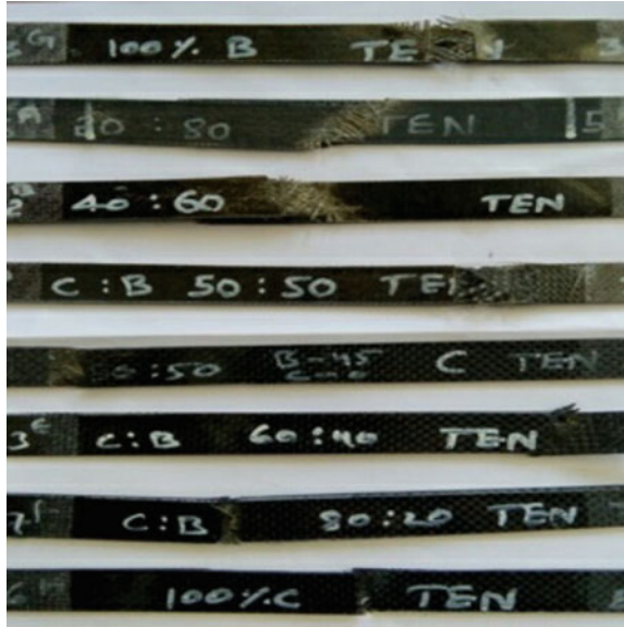
Fig. 61.3 Fractured samples after tensile test
