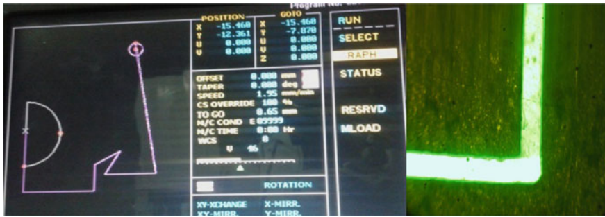
Fig. 47.2 Cutting rate and kerf width measurement
