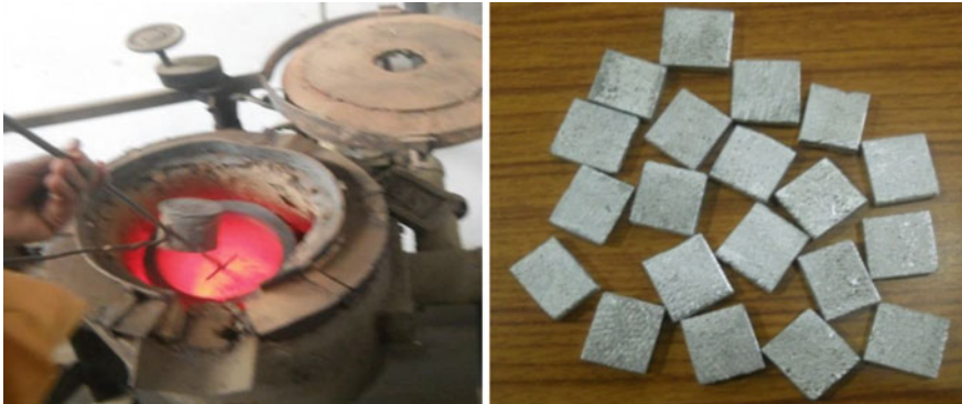
Fig. 30.1 Specimens prepared via stir casting method
