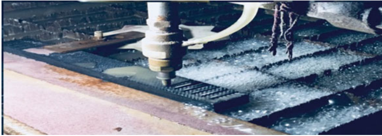
Fig. 52.1 Machining of carbon fibre vinyl ester composite by AWJM
