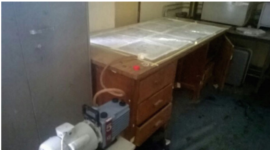
Fig. 61.2 Experimental setup of vacuum bagging
