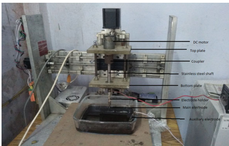
Fig. 7.2 Photograph of experimental setup
