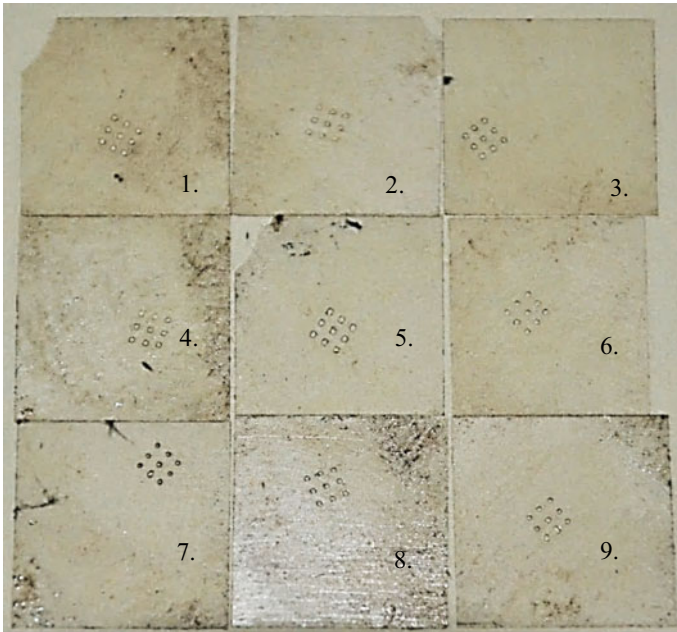
Fig. 45.3 The drilled glass samples after experimentations
