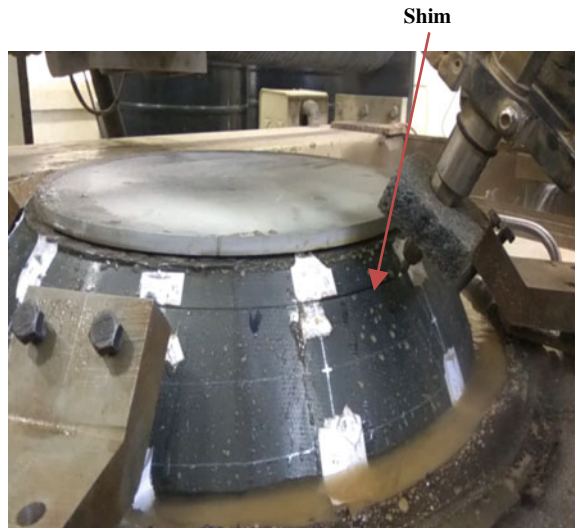
Fig. 34.8 AWJ cutting of shim
