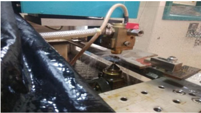
Fig. 32.2 Clamping of SS 316L on WEDM
