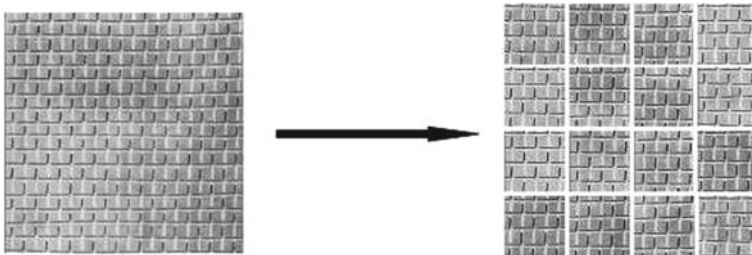
Fig. 2 Example of images (D1) from Brodatz album divided into 16 equal subimages for database creation
