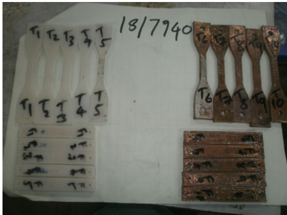
Fig. 25.7 Electroplated and non-electroplated specimens
