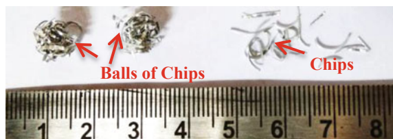
Fig. 34.1 Chips compacted into ball-shaped structure
