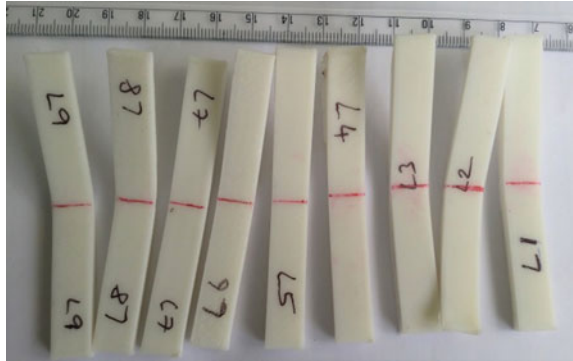
Fig. 20.2 Fractured specimens after flexural test
