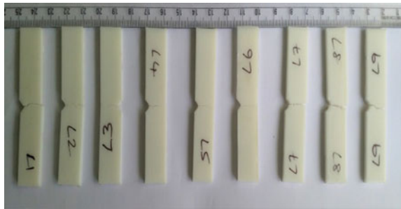
Fig. 20.3 Fractured specimens after impact test
