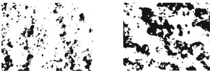
(a) Conventional Sand Mold (b) Orange Peel Activated Layered Mold
