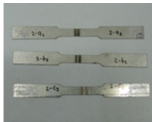
Fig. 39.2 Tensile sample dimension as per ASTM-B557M-10
