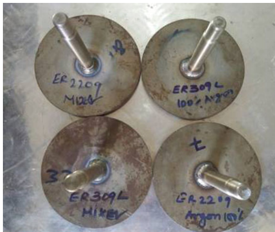
Fig. 47.2 Push rod assembly welded with different filler wires and gas mixtures
