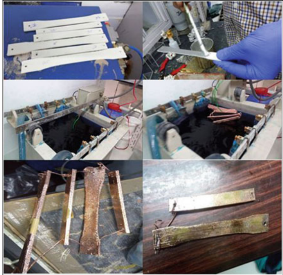
Fig. 25.6 Electroplating of 3D-printed HIPS specimens
