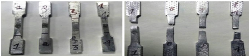
Fig. 44.9 Tensile test specimens before and after fracture
