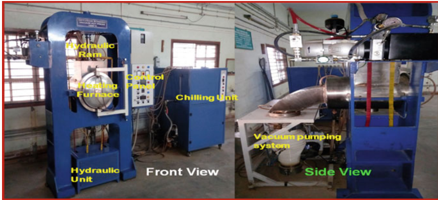
Fig. 66.1 Diffusion bonding machine setup
