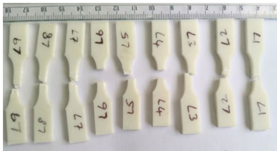
Fig. 20.1 Fractured specimens after tensile test
