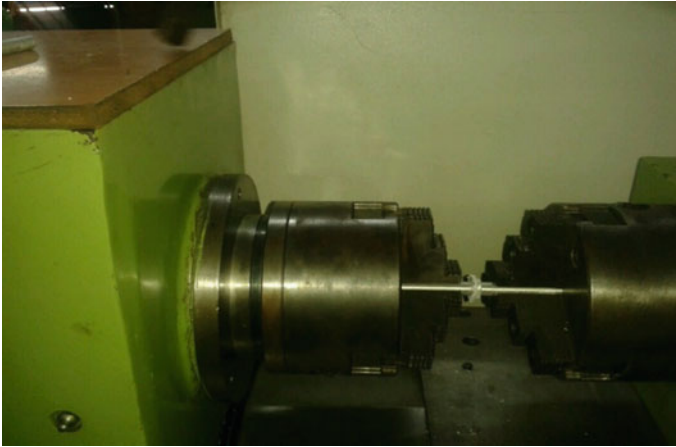
Fig. 65.2 Friction welding machine set-up
