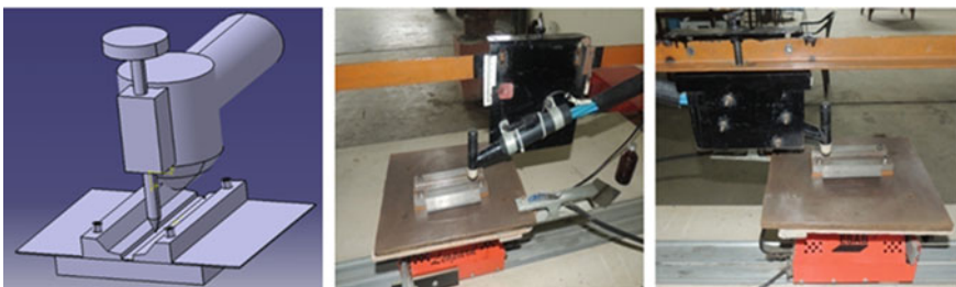
Fig. 39.1 Modified and fabricated fixture
