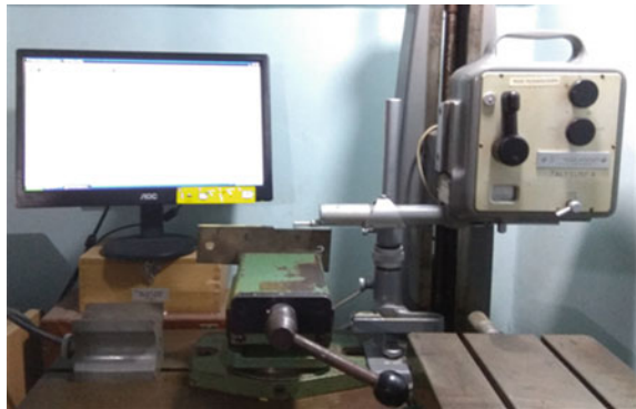
Fig. 42.3 Taylor Hobson Talysurf setup and profile of surface roughness
