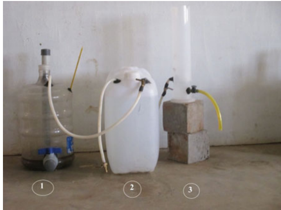
Fig. 1 Anaerobic digester fed with inoculums
