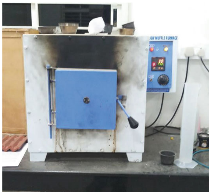
Fig. 3 Placing the poultry sample in the muffle furnace for proximate analysis
