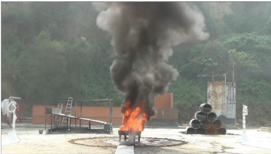
Fig. 6 Observations of explosive burning with perlites
