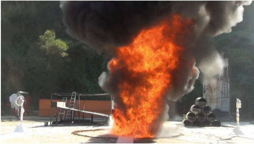
Fig. 5 Observations of explosive burning without perlites
