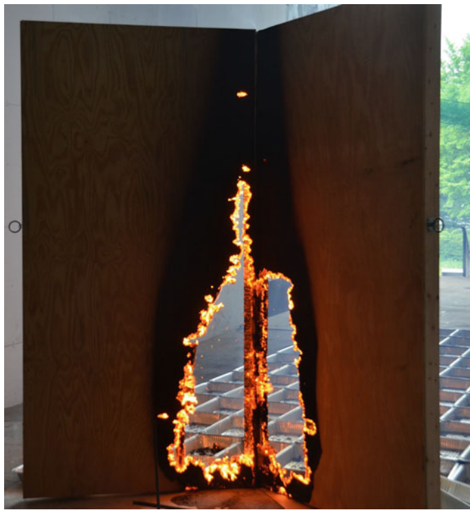
Fig. 2 Full-scale re-entrant corner ignited and 8 m/s wind has been applied. The water pan array is used to collect the firebrands produced
