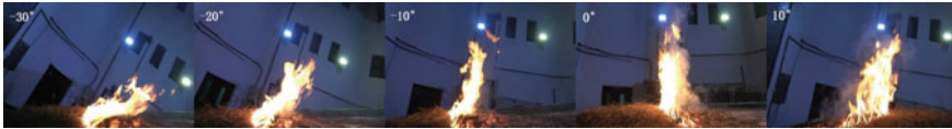
Fig. 2 Flame geometry for tests with variable slope from -30^\circ to 10^\circ . Note that the camera was bound to the bench
