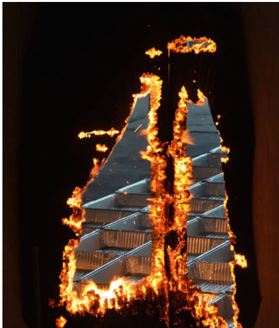
Fig. 5 Picture of firebrand generation process for a wind speed of 8 m/s. The combustion of plywood and wood studs may be observed
