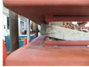
(b) 1-t60-400 Rotational displacement at the supporting part
