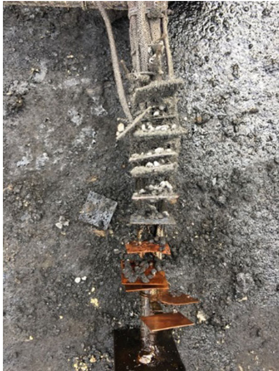
Fig. 9 Thermocouples were stuck by perlites
