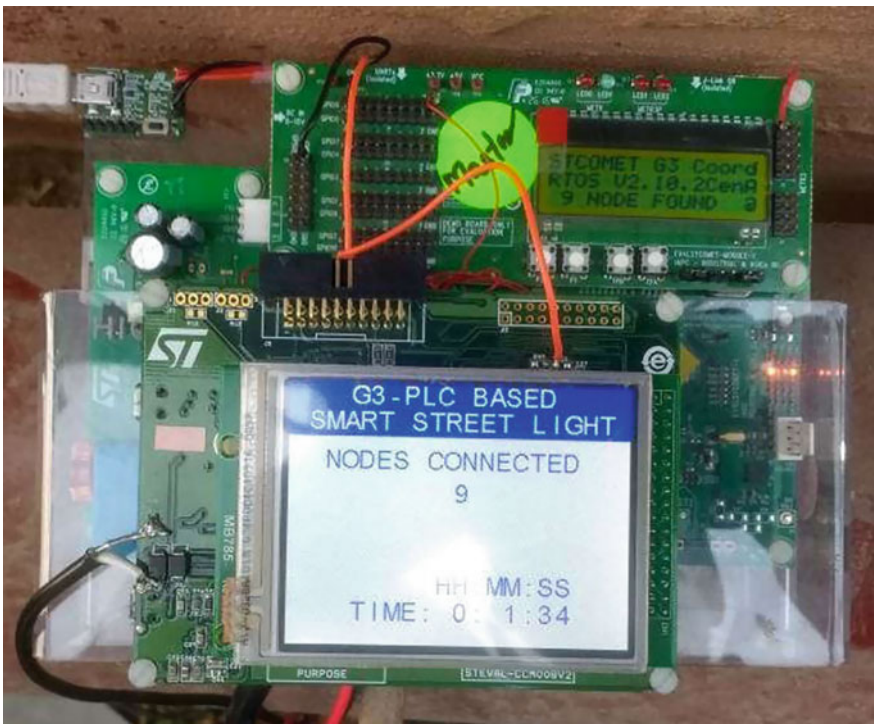
Fig. 3 DCU of G3-PLC based LED streetlight
