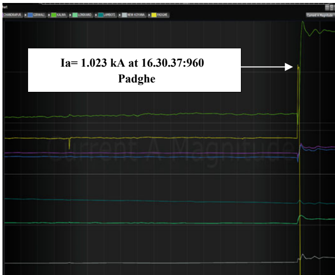
Fig. 10 A-phase current rise during second fault at 400 kV Padghe substation
