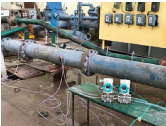
Fig. 9.2 Layout of sloped downstream large pipeline with by-pass line
