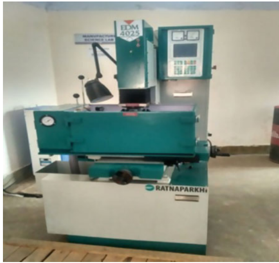
Fig. 8.1 Sinker EDM apparatus used for the experiment
