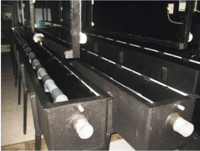
Fig. 10.7 Prototype of raceway system for larval culture of Thenus unimaculatus at Field Laboratory of CMFRI at Kovalam, Chennai, India
