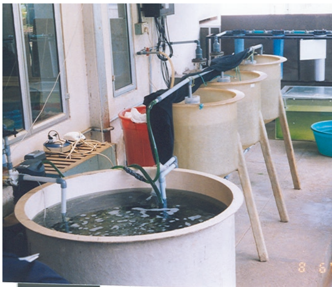
Fig. 10.3 Clear water recirculation system for culturing phyllosoma larvae of Panulirus homarus homarus at CMFRI, Kochi, India. (Photo by: E. V. Radhakrishnan, CMFRI)
