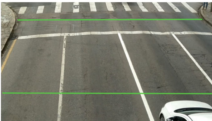
Fig. 5 Reference lines for estimating the speed
