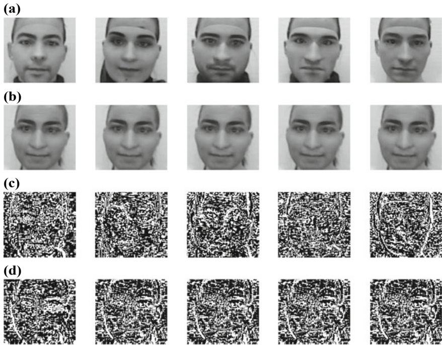
Fig. 2 a Low rank/Diffused component of spoofed faces wearing 3D masks; b Low rank/Diffused component of real legitimate faces; c Sparse/Specular component of 3D mask faces; d Sparse/Specular component of real genuine faces
