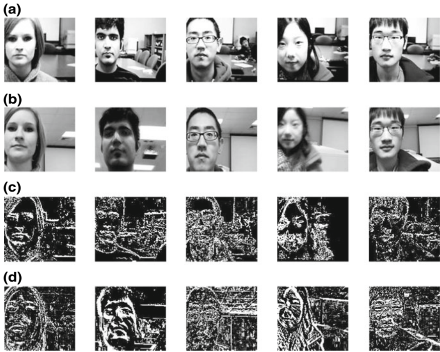
Fig. 1 a Low rank/Diffused component of attack face especially printed photo attack faces; b Low rank/Diffused component of real legitimate faces; c Sparse/Specular component of printed photo attack faces; d Sparse/Specular component of real genuine faces. Images are taken from Wen et al. [9] printed photo database
