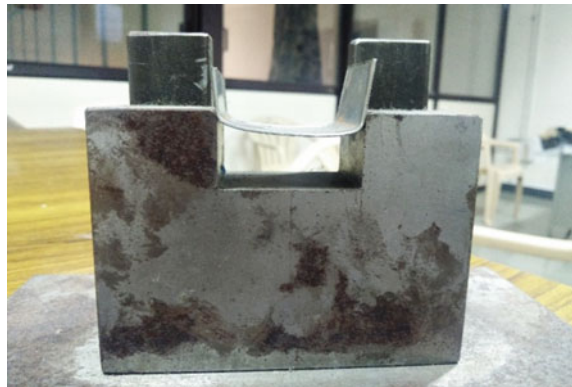
Fig. 7.2 Experimental setup for U-bending
