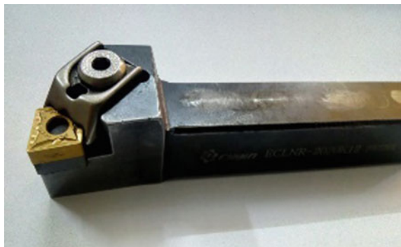
Fig. 27.5 Cutting inserts and tool holder
