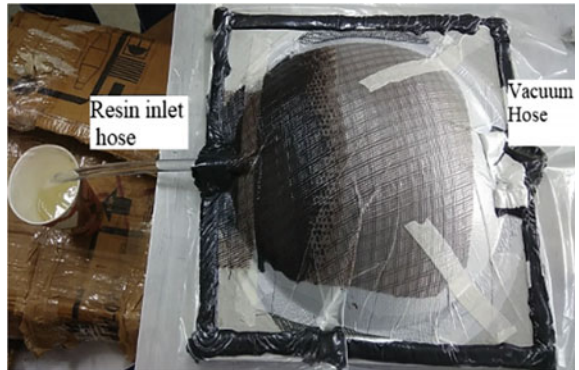
Fig. 58.7 Resin inlet hose and vacuum hose
