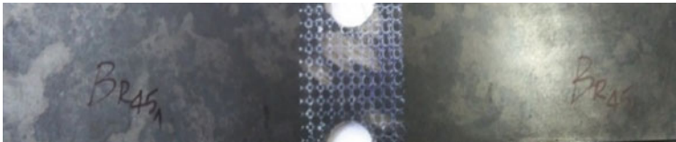
Fig. 3.3 Typical plane-strain tension specimen before test
