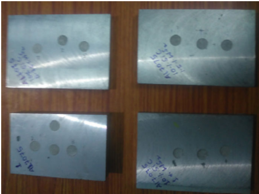
Fig. 28.1 Samples machined on EDM machine
