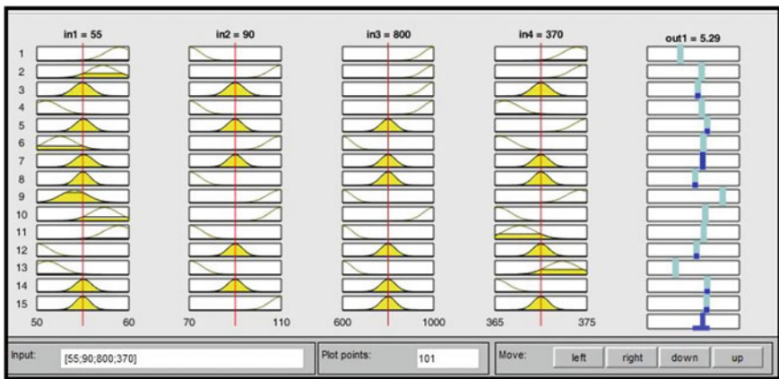
Fig. 70.2 Updated rule base for a specific input data combination [55, 90, 800, 370]
