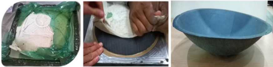
Fig. 58.10 Autoclave demoulding process and cured reflector
