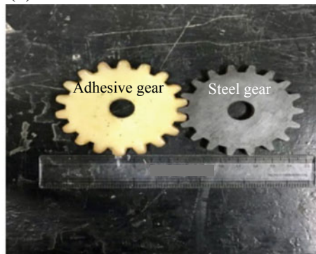
Fig. 77.3 a Making of adhesive gear using mould and b fabricated adhesive gear and steel gear
