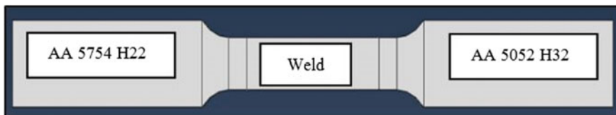
Fig. 2.5 TWB tensile specimen modeled in ABAQUS
