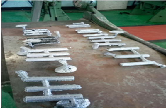
Fig. 62.2 Manufacturing of Al/SiC-bagasse ash composite
