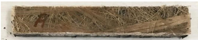
Fig. 64.3 Sample for flexural testing as per ASTM D790
