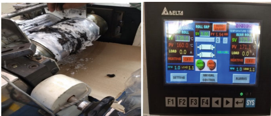
Fig. 65.1 Mixing of fibers with polypropylene in two-roll mill
