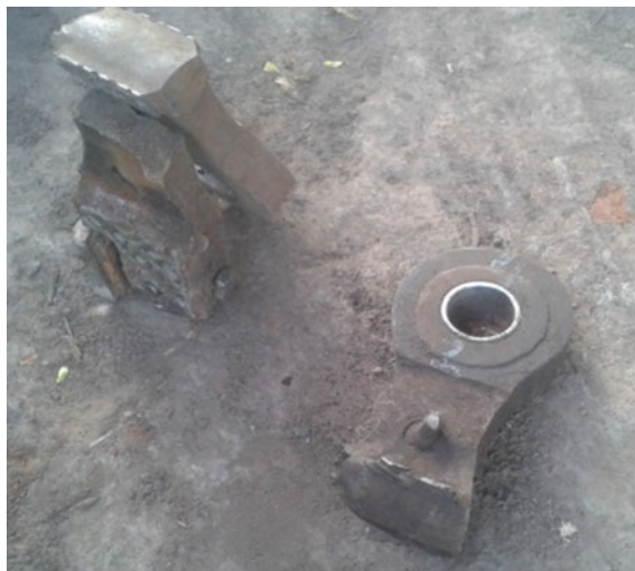
Fig. 78.4 Broken parts of Fibrizer hammer
