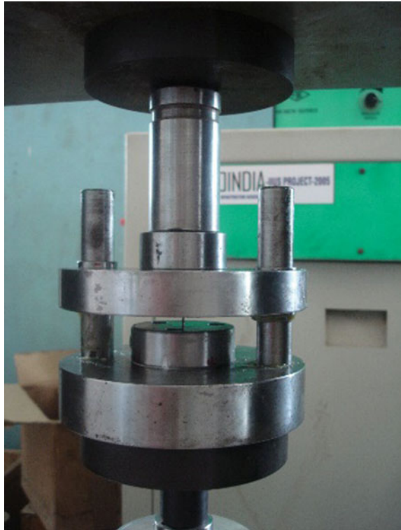
Fig. 1.4 Micro extrusion—die assembly
