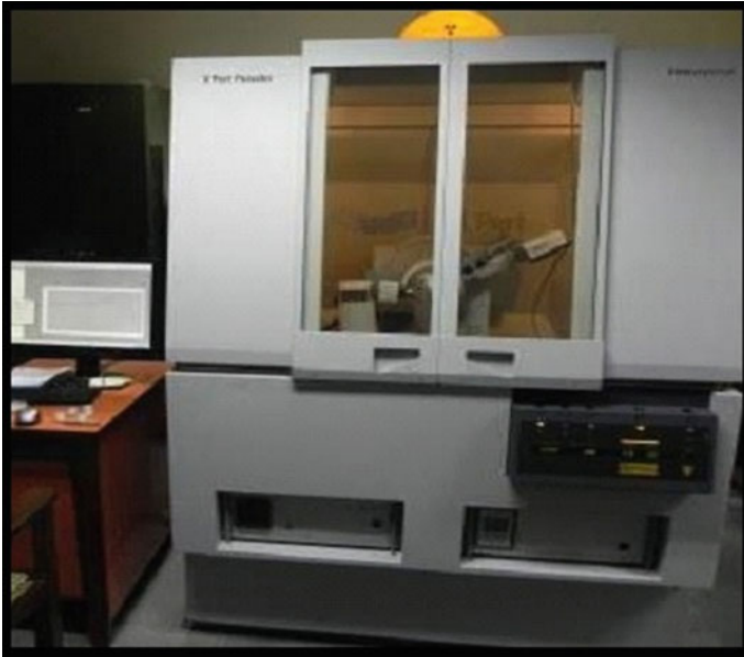
Fig. 9.4 GIXRD Panalytical™ set-up (Courtesy IIT, Bombay)
