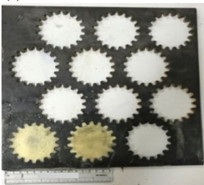
Fig. 77.3 a Making of adhesive gear using mould and b fabricated adhesive gear and steel gear
