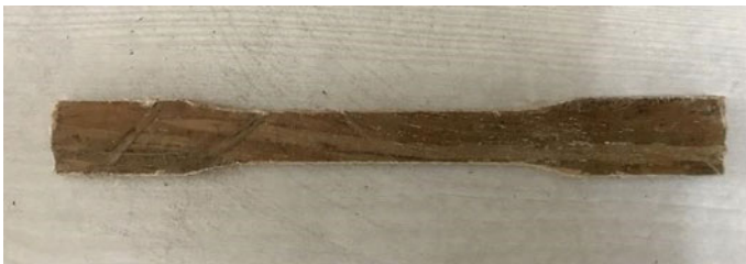
Fig. 64.2 Sample for tensile testing as per ASTM D638
