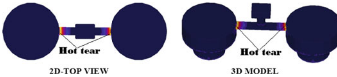
Fig. 40.7 Hot tear region of Al–Cu cast alloy: 2D-top view and 3D-model
