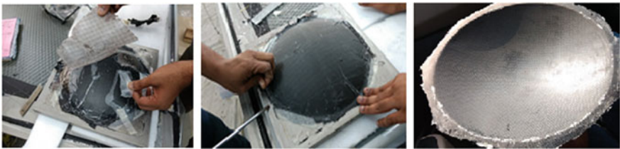
Fig. 58.11 VARTM demoulding process and cured reflector
