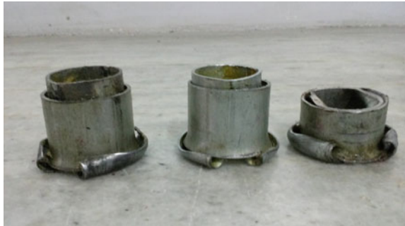
Fig. 6.9 Joints made by end forming
