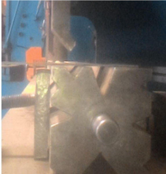
Fig. 8.2 Experimental setup for V-bending
