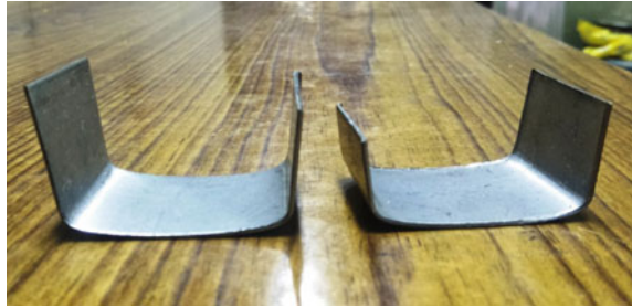
Fig. 7.3 Deformed images after forming the sheet metal
