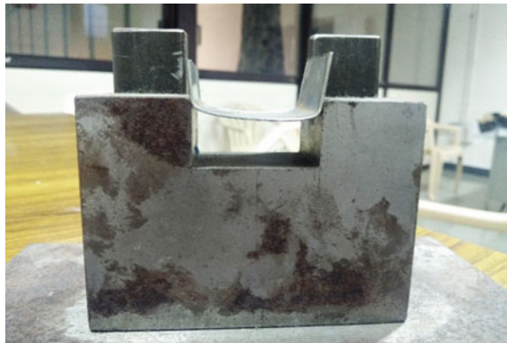
Fig. 7.2 Experimental setup for U-bending
