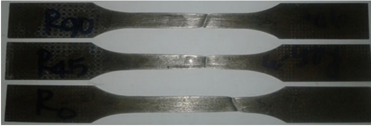
Fig. 3.5 EN-10149-2 specimen after tensile test
