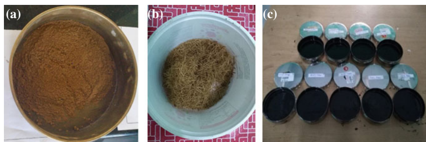
Fig. 1 Materials used a Coir powder b Coir fiber c Bitumen
