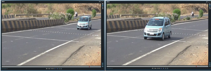
Fig. 1 Car tire touching the first and second line of trap length
