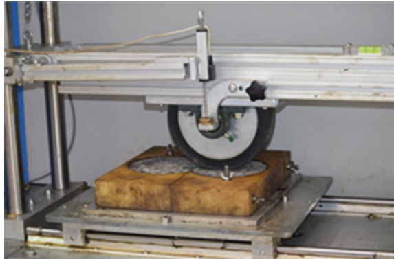
Fig. 3 Experimental setup of wheel-tracking test
