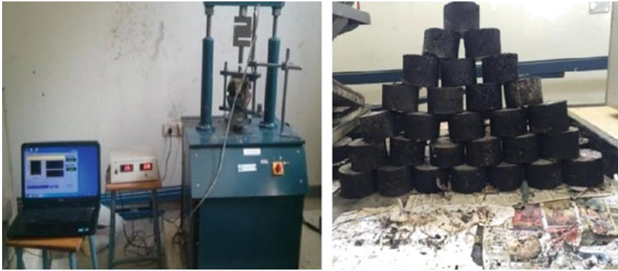
Fig. 3 Marshal setup with specimens
