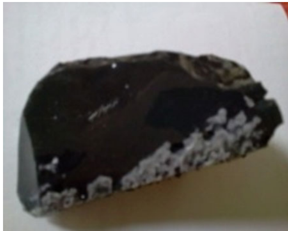
Fig. 38.3 Appearance of the melt from technogenic waste and broken glass with a mass content of components 50:50 (waste: cullet)
