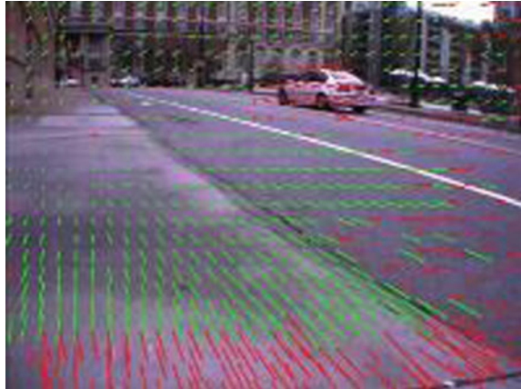
Fig. 5.2 Vector arrangements of optical flow
