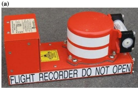
Fig. 32.1 a Cockpit audio voice recorder unit of an airplane. b Flight data recorder of an airplane. c Voyage data recorder for sea vessel
