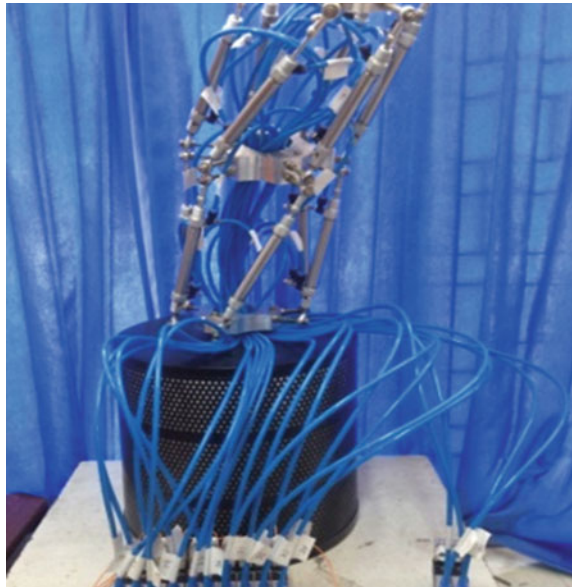
Fig. 4.2 Implementation of Discrete Manipulator with 12 Discrete Actuators
