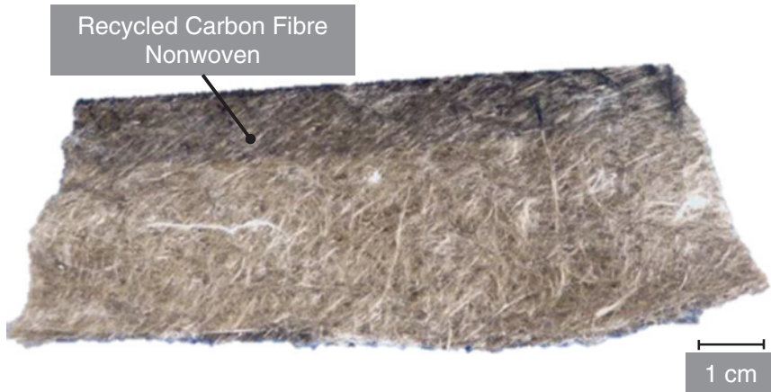
Fig. 12 Coated recycled carbon fibre nonwoven [30] (Source ITA)
