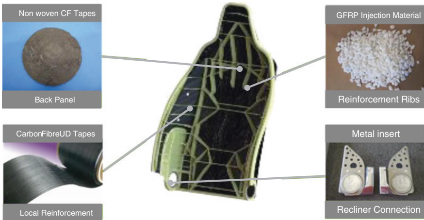
Fig. 14 Depiction of a seat back in CAMISMA’s material mix approach with specific depiction of the recycling material [23] (Source JCI)
