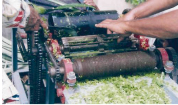
Fig. 15 Scrapping machine of pine leaves [50]
