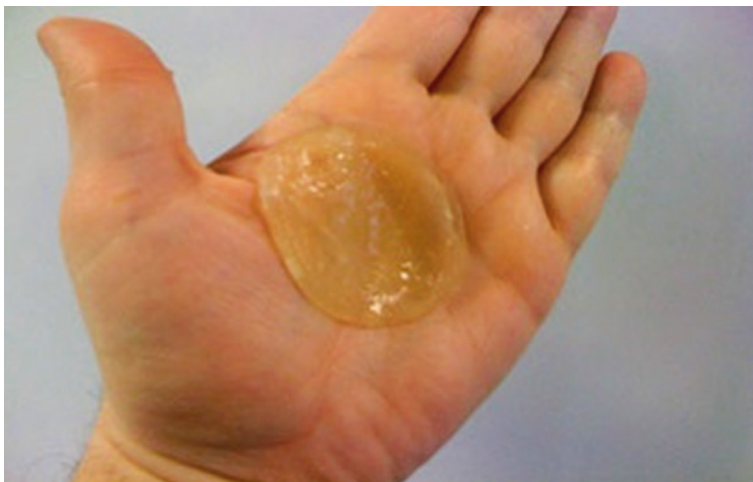
Fig. 4 A prototype mucilage/gelatin hydrogel patch (© Spring 2012, with kind permission of Dr Iain Allan, School of Pharmacy and Biomolecular Sciences, University of Brighton, UK)
