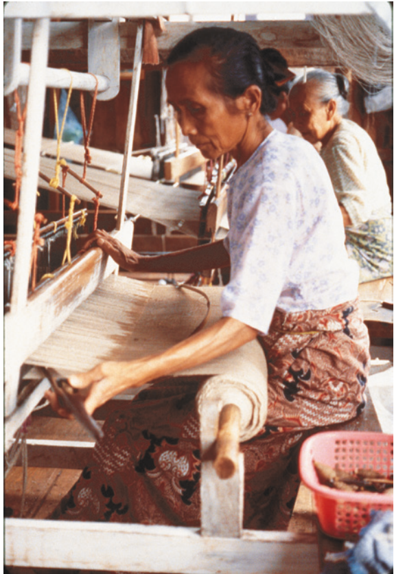
Fig. 4 Manually weaving the lotus fiber yarn. Source Fraser-Lu and Thanegi [11]. Photograph by Sylvia Fraser-Lu, Pandonmar Lotus workshop, Kyaing-kan, In-le, 2000. Published with the authorization of Sylvia Fraser-Lu and the Fowler Museum at UCLA
