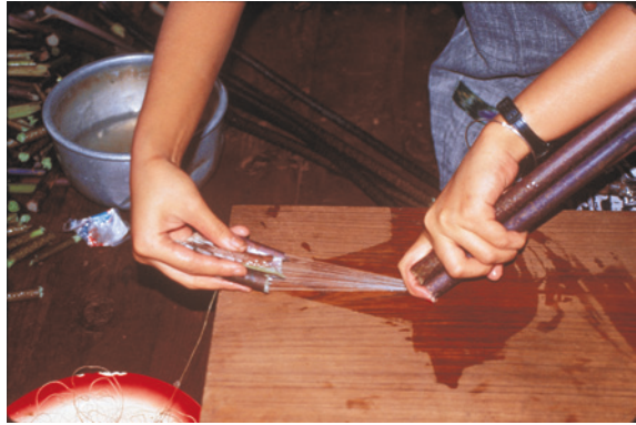
Fig. 1 Obtaining the fibers from the lotus flower stem. Source Fraser-Lu and Thanegi [11]. Photograph by Sylvia Fraser Lu, Pandonmar Lotus workshop, Kyaing-kan, In-le, 2000. Published with the authorization of Sylvia Fraser-Lu and the Fowler Museum at UCLA
