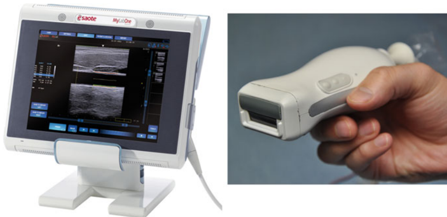
Fig. 9 Portable system combining ultrasound and photoacoustics. Left is the US scanner and right shows the photograph of probe combining laser module and ultrasound transducer array. (Reprinted from Ref. [36]. With permission from the authors and Optical Society of America)
