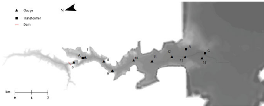
Fig. 1 Malpasset test domain with location of the transformers, the 9 gauges along the Reyran valley and the dam
