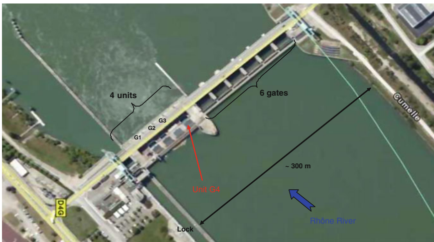
Fig. 2 Plan view of Vaugris hydropower plant
