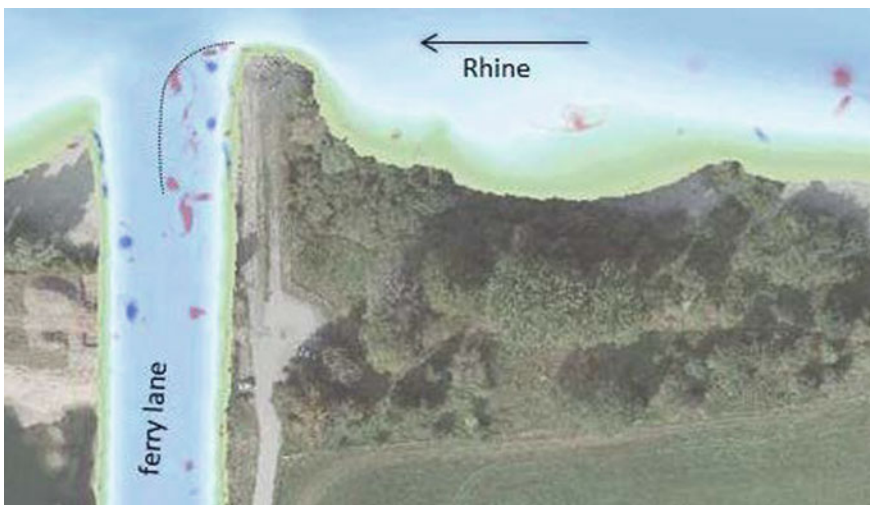
Fig. 6 Eddy motion of the flow simulation in the ferry lane opposite Rees
