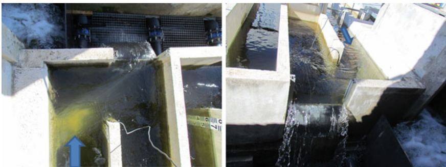
Fig. 1 PAC-UPC laboratory canal bend in operation
