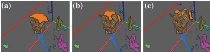
Fig. 3 Pore shape variation within XY plane at a slice 100; b slice 105; and c slice 110
