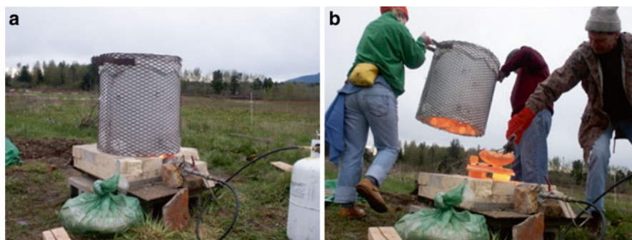
Fig. 17.2 (a) Modern raku kiln. (b) Lifting up the raku kiln to take out fired pieces (Oten Pottery, 2007)
