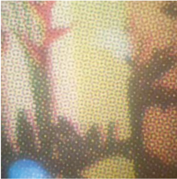
Fig. 4.1 Example of the offset lithography examination (the dots are arranged in regular rows and column)
