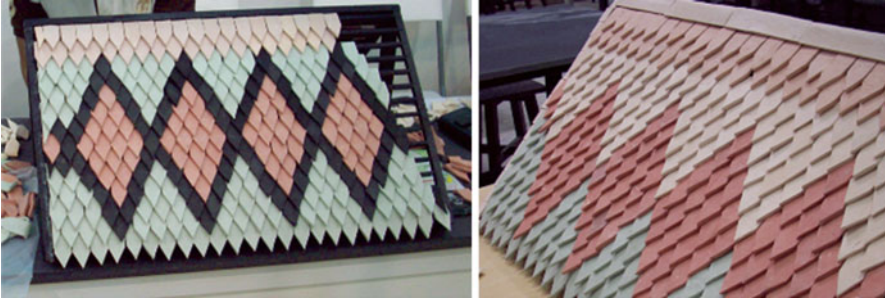
Fig. 66.8 Prototype of the new Singgora in modern architecture – gazebo (Patent pending)
