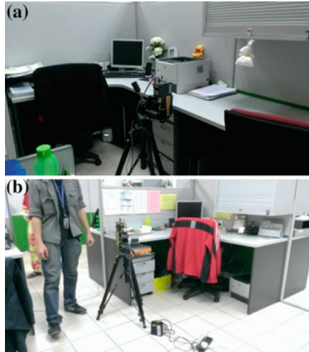
Fig. 3 a Laser Doppler vibrometer (LDV 100). b Measurement at site
