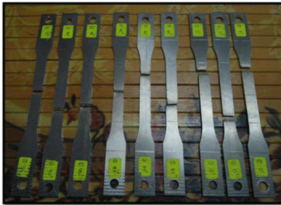
Fig. 10 The tensile fracture of AA5083 specimens
