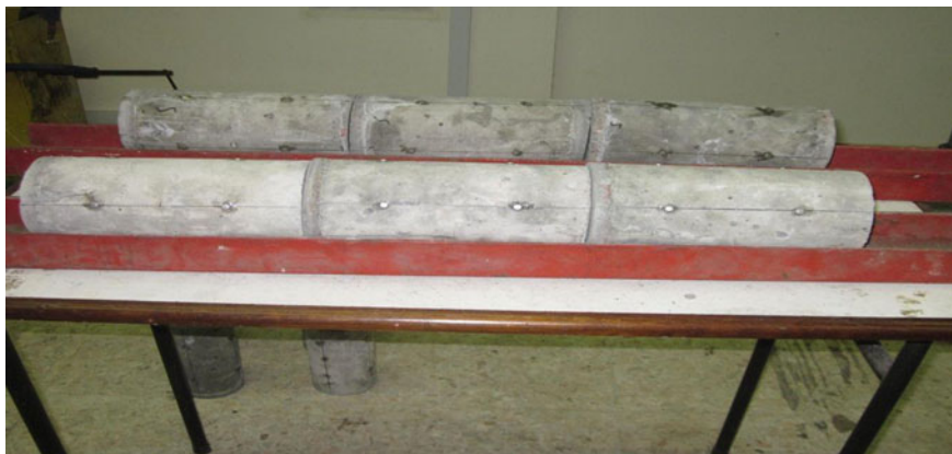
Fig. 2 Sample preparation for creep and shrinkage
