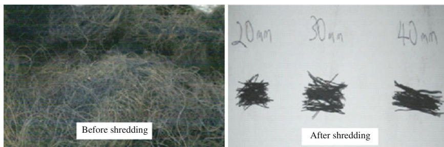
Fig. 1 Recycled steel fibre before and after shredding
