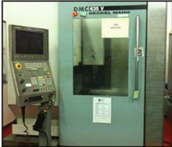
Fig. 4 CNC milling machine that was used to cut the specimens into dog-bone shape
