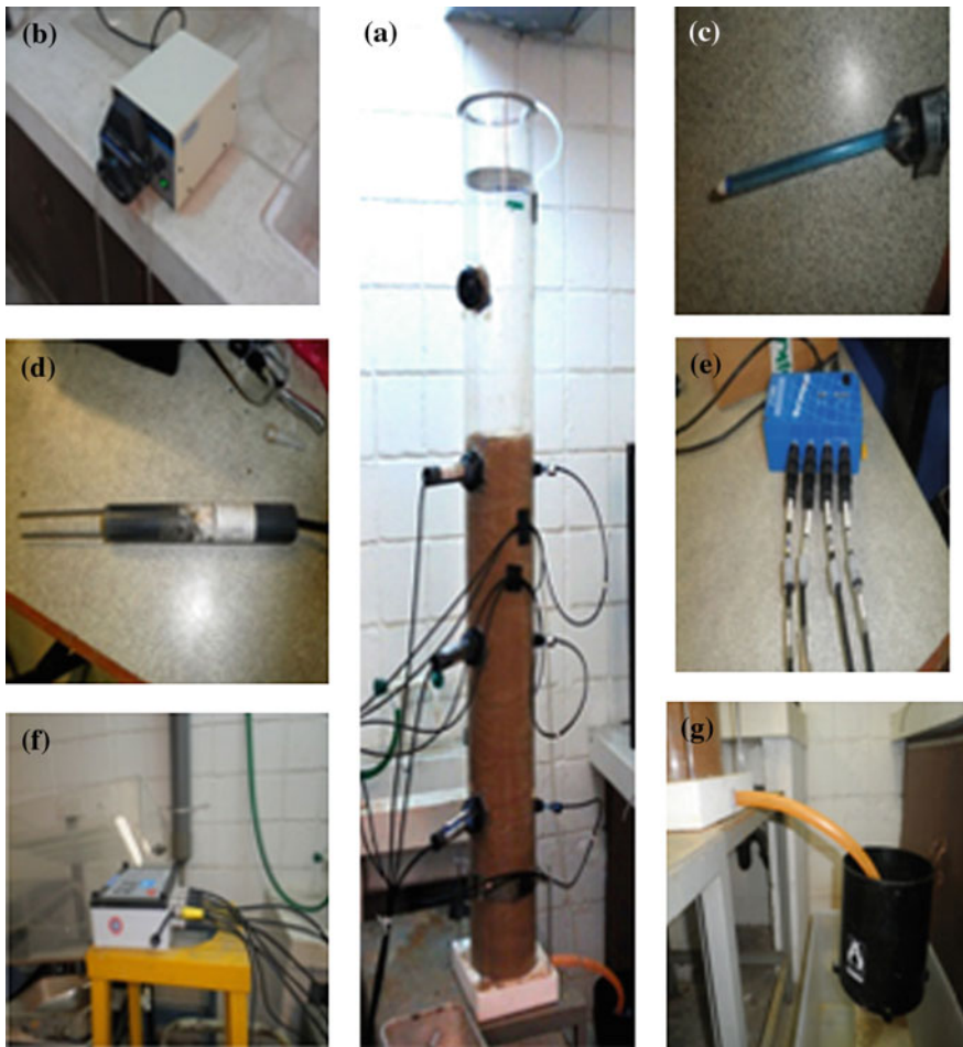
Fig. 2 Soil column apparatus a Soil column cylinder b flow regulator c tensiometer d TDR e data logger for TDR f data logger for tensiometer g effluent rain gauge
