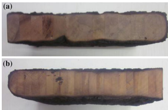
Fig. 7 Charred cross-section of glulam after 1 h exposure; a keruing and b malangangai
