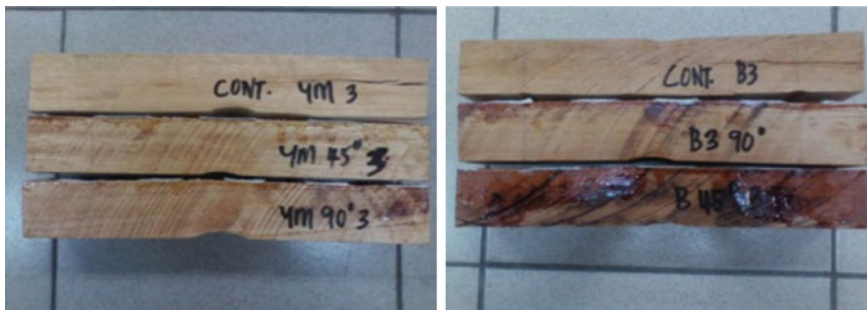
Fig. 9 Mode of failure between Yellow Meranti and Bintangor specimen
