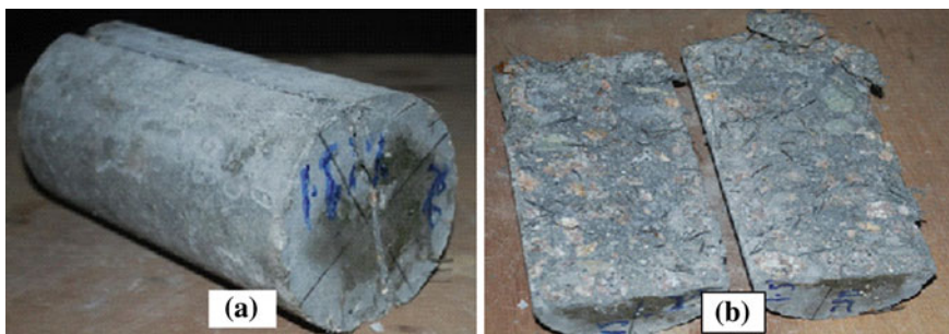
Fig. 5 a Concrete cylinder after splitting tensile test. b Distribution of steel fibre in broken cylinder
