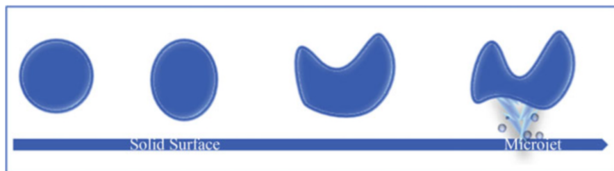
Fig. 3 The occurrence of transient cavitation near a solid surface and the resulted asymmetrical bubble collapse and the generation of liquid micro-jets [36]
