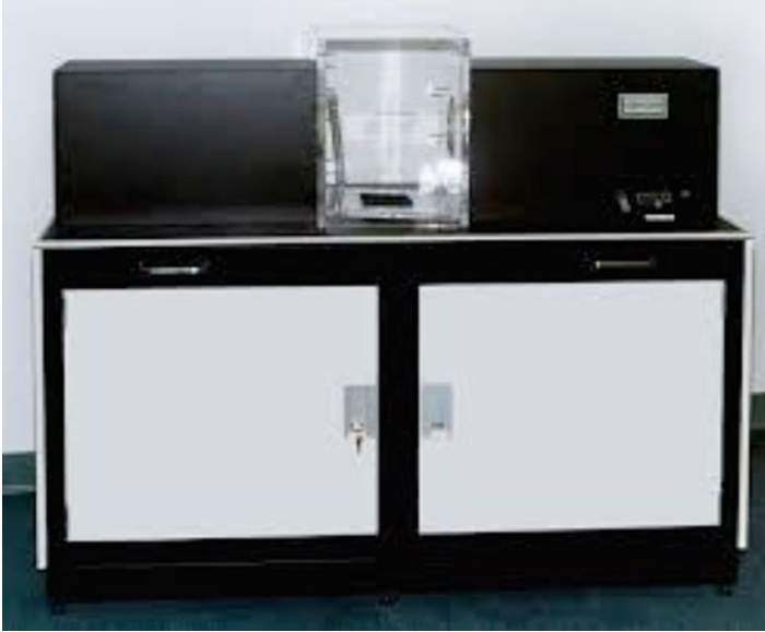
Fig. 10 Commercially available quantitative stroboscopic Schlieren system designed for visualization of both continuous and pulsed ultrasound fields ( http://www.ondacorp.com/products.shtml , accessed Aug. 26, 2015)
