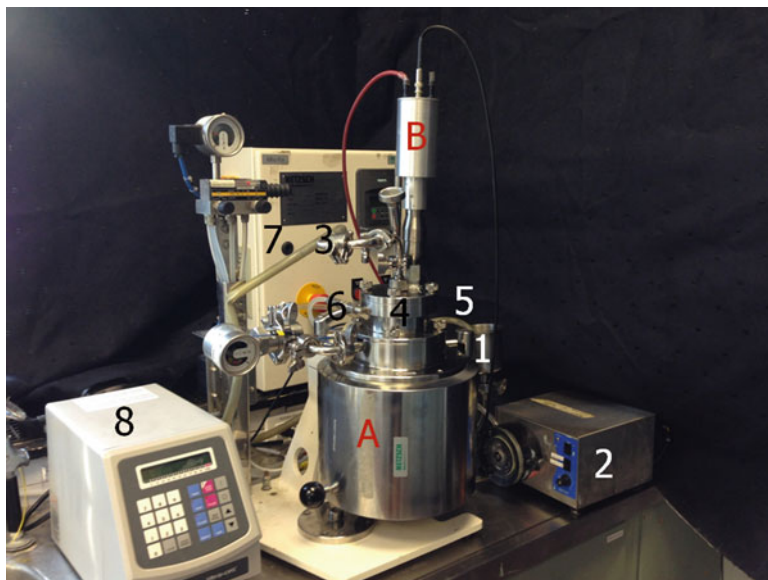
Fig. 2 Mini-fer (Netsch) ball mill with an ultrasonic horn. (a) Ball mill (b) direct sonicator – ultrasonic horn (1) feed tank (2) feed pump (3) charging point (4) mixing chamber (5) discharging point (6) cooling water (7) micronizer motor (8) ultrasound control (Reprinted with permission from [29]. Copyright 2015 AIDIC)
