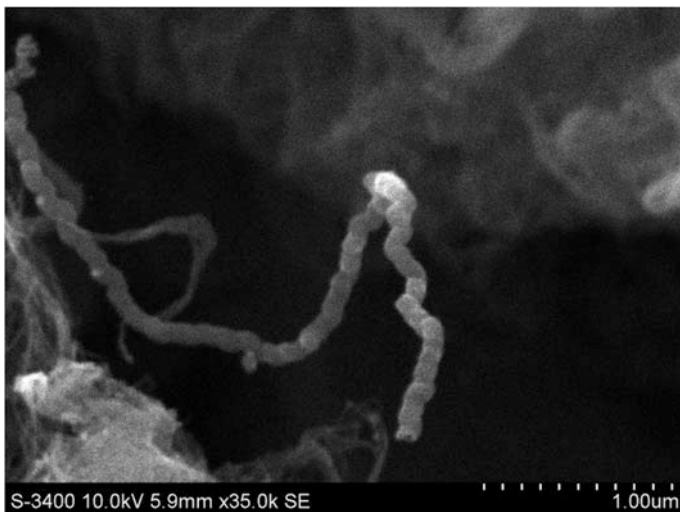
Fig. 3 SEM Image of purified SWCNT sample produced by the HiPco technique
