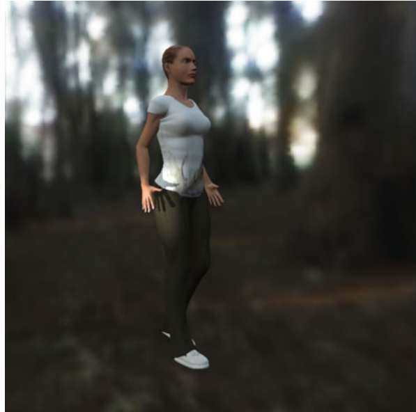
Fig 4.10 Our real-time, skinned virtual character along with spot-based lighting, image-based lighting, ambient occlusion, shadow mapping, subsurface scattering, and environment mapping
