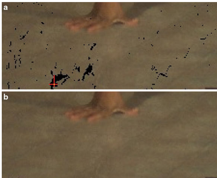
Fig. 11.3 (a) Generated view with void pixels (one of the pixels to be interpolated is in yellow , and the directions of search for pixels to be used in bilinear interpolation are in red ) and (b) interpolated void pixels using the proposed algorithm
